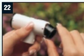
22 Glues into 1/2" slip PVC fitting; accepts [40] 1/2" drip tubing (.7" O.D.)
